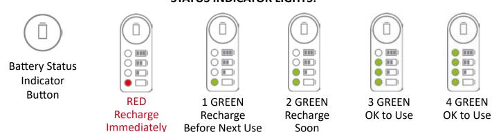
**WARNING:** The battery must be put on charge immediately as soon as the red indicator light appears. Running the Airflo 12 on RED until the battery is exhausted will damage the battery.
