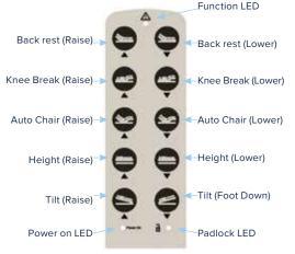
When the power is connected, the power LED illuminates. The function LED illuminates when a function button has been pressed.
