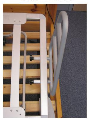
When fitting the Side Rail for a slatted bed, the threaded rods should first be introduced to the trombone, then the spacers put onto the rods and finally the hand wheels tightened until a firm fitting is achieved. This will allow the Side Rail to fit inside the frame of the bed in its lowest position.
