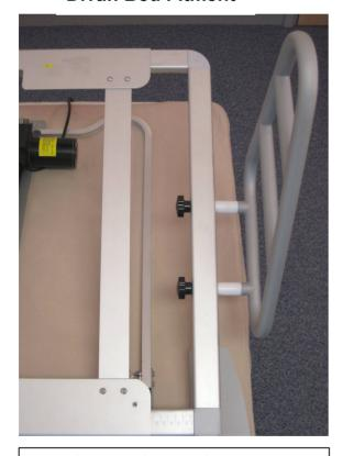
When fitting the Side Rail for a divan bed, the spacers should be put onto the threaded rods before they are introduced to the trombone. The hand wheels should then be tightened against the inside of the trombone until a firm fitting is achieved. This will allow the rail to be on the outside of the mattress.
